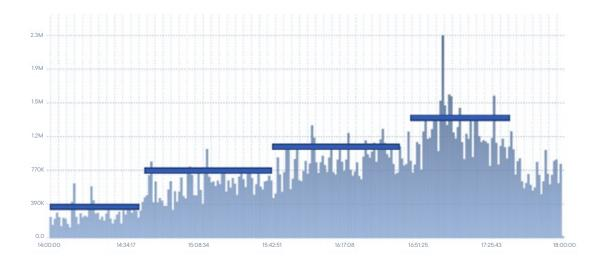
The four blue lines indicate an incremental growth of the traffic volume: from ~400K packets to ~1.35M over 3 hours (with a significant spike of 2.3M). Incremental growth like this is very common in DDoS attacks, where various attacking bots "wake up" on a delay from each other (in order to allow them to blend in with regular traffic) and begin to bombard the network, one after the other—until they all bombard it together, which eventually causes it to crash.
